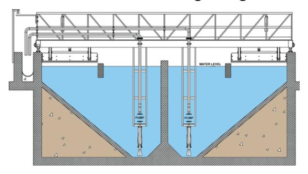
The grit and grease travelling bridge KD 22 consists of a complete travelling bridge with separate drive unit, mechanical surface scrapers for collection of surface sediment and submersible pump unit (optional) for collection of settled grit.
