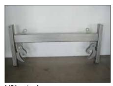
*Lifting tool.* By using sectional Stop Logs and our specially designed lifting
