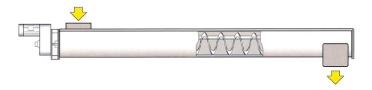
**Shaftless Screw Conveyors KD 02** are available in four sizes with capacities from 5 to 20 m<sup>3</sup> per hour. The conveyors are especially suited for products with a tendency towards tackiness and bridgebuilding e.g. sludge, damp sand and materials with heterogeneous grain sizes.
