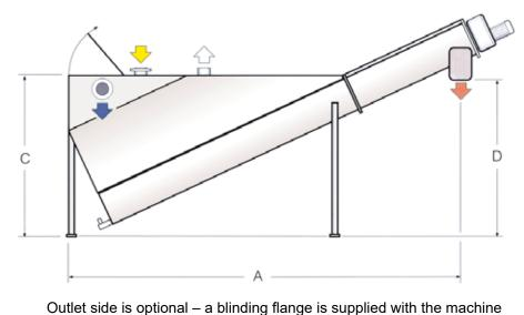
The Grit Classifier KD 01 is available in five sizes with a separating capacity from 20 to 140 m<sup>3</sup>/h. The separator is constructed in stainless steel and after machining completely pickled. By this, the optimal durability of the material is ensured.
